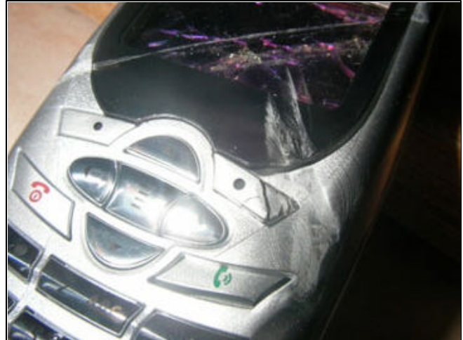
Small cracks and abrasions form of the face of a cordless phone when it is hung up in a smashing action.
